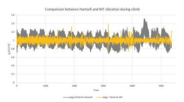
Vibration performance obtained through our own instrumented flight tests
